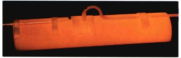
Thermocouple testing at 2100°F. The thermocouples are mounted on a boiler tube shield; the thermocouple on the left is measuring temperature near the tube shield; the (tubeskin) thermocouple on the right is directly measuring tube shield temperature.
